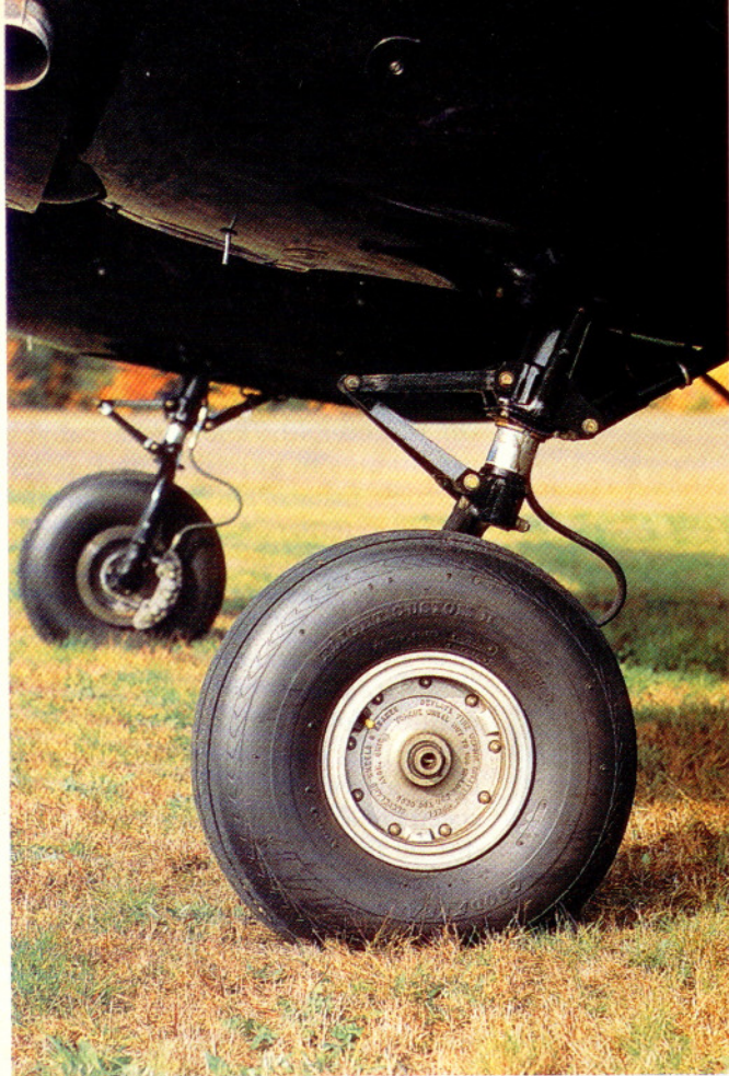
The main landing gear retracts via a bicycle chain and worm gear arrangement (left). There's seating for three across on the rear bench (opposite).
